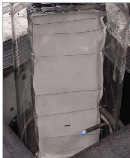
KYNAR® PVDF foams are tested to FM 4910 using the Fire Propagation Apparatus.
